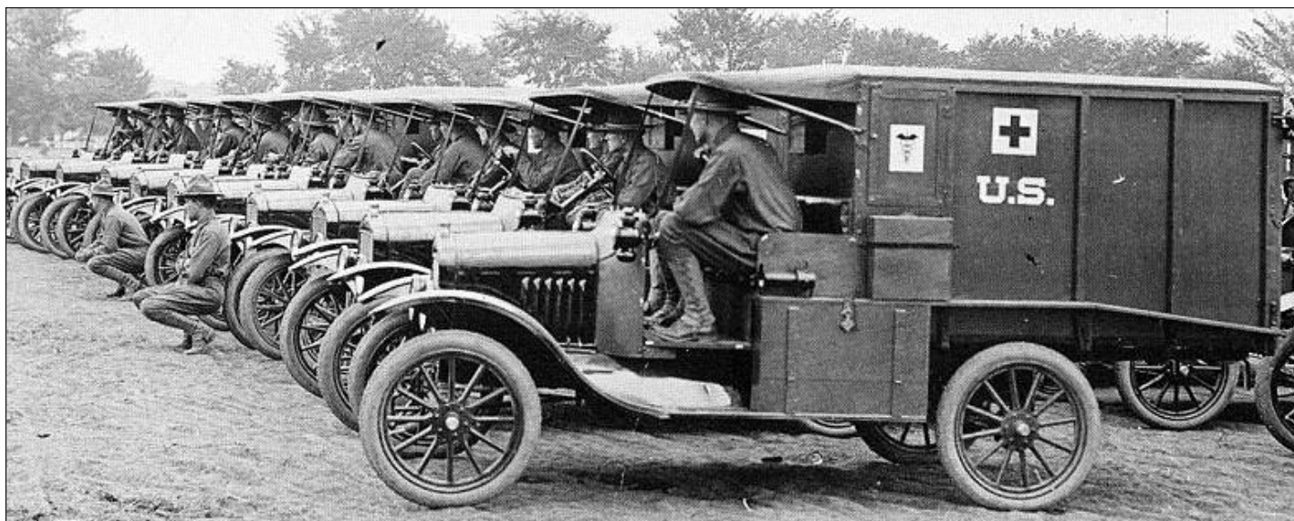
A lineup of M-17 Ford Model-T ambulances at Camp Crane in Pennsylvania, 1917. It could carry three patients on stretchers or five in a sitting position. (U.S. Army)
